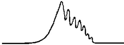
This crystal ringing can be cleaned up by adjusting the phasing capacitor C75 until the best symmetrical curve is obtained. Once this has been completed adjustment of the bottom cores of the I.F. transformers and C80, C81 (similar in type to those in the R.F. stages and located near C75) can be commenced until all selectivity positions have response curves as near to the ideal as possible.
