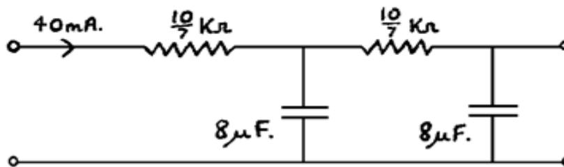
What of the voltage drop and power dissipation of this arrangement?
