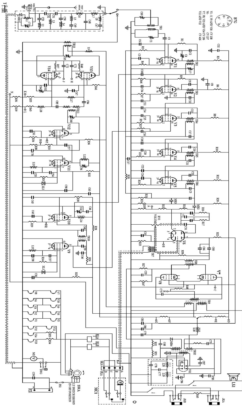
Fig 1001 - W.S. B44 MR 2 - circuit diagram
