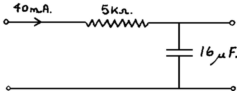
If we have a full wave rectifier circuit followed by an R/C filter with the typical values shown, this filter will reduce the 100c/s ripple from the rectifier as follows :-
