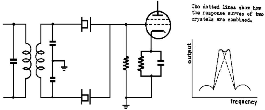
FIG 6 HALF LATTICE FILTER WITH SHUNT CRYSTALS
