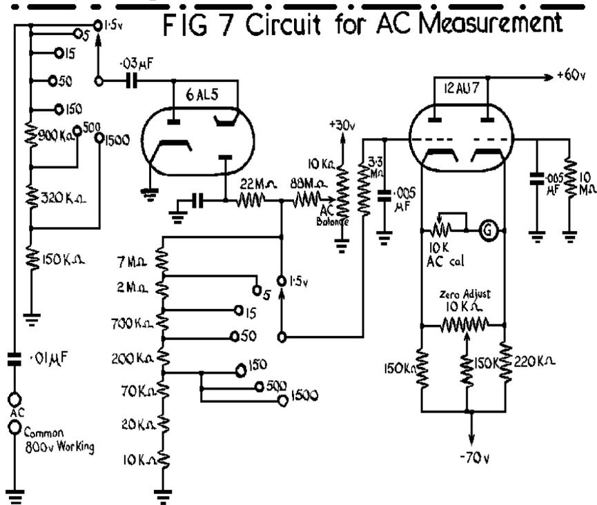
Component values are given so that this can be reproduced if desired. It was, in fact, described in Electronic Engineering for January 1950. It is built round a 500 microamp surplus meter. The scale reads DC and peak AC volts.
