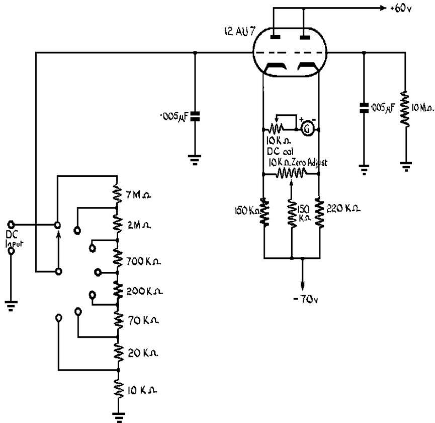
FIG 7 Circuit for AC Measurement
