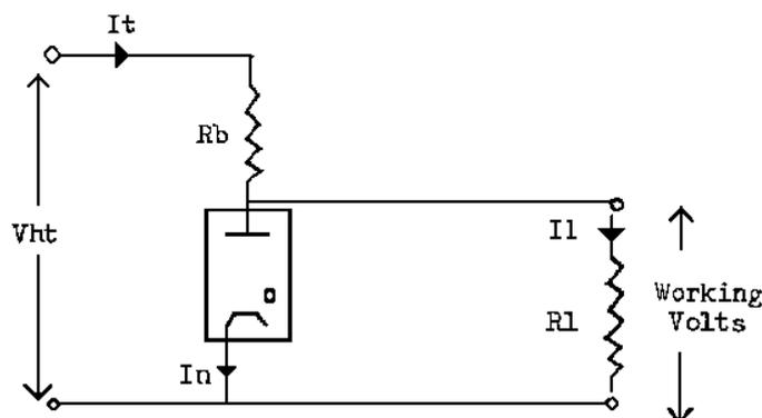
The function of the series resistor  $R_b$  is to limit the current flow when the neon strikes. If it were not there the current would increase to such an extent that the neon would be destroyed.
