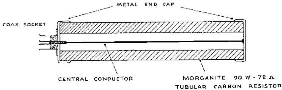
FIG 4. 72  $\Omega$  NON-INDUCTIVE LOAD.
