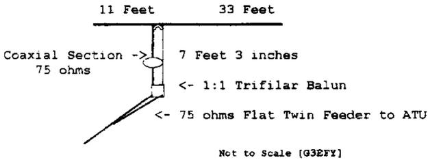
Fig 3. Suggested Modified Trap Dipole to include a vertical radiator
