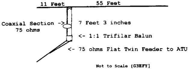
Fig 2. 21 MHz Monoband Antenna One Wavelength.
