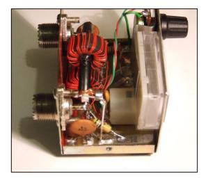
The two SO239 sockets are connected using a short piece of 50? coax which is connected only to ground and the Bremi chassis at one end. This can be seen as the long silver plated vertical wire in the photo. The coax is inserted into the voltage transformer and is later secured with clear contact adhesive.
