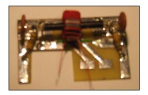
The coupler PCB with the measuring line installed. Two pieces of stiff silver plated wire were used to create "L" shaped supports at each of the 50? coax. The bottom of each is soldered to each of the shorter copper lands on the PCB, creating a short metal support, used to solder together the two resistors, the decoupling capacitor and diode. The wires should be long enough to support the 50? coax so that it passes centrally through the toroid.
