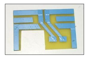
The new coupler glass fibre PCB replaces the original circuitry inside the Altai SWR meter. It also requires a cut-out so that the PCB can slide under the front panel meter. It is relatively simple to make using a junior hacksaw, a metal file, electrician's insulation tape and bath of ferric chloride. See details below.
