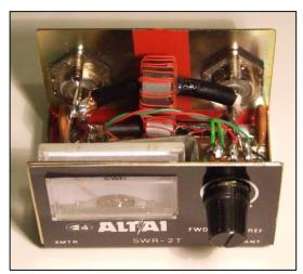
The photo shows the front view of the SWR meter after modification and the red and green wires that provide the forward and reverse voltages to the calibration potentiometer via the FWD-REF switch underneath the knob.
