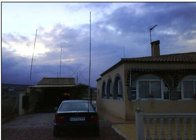
The 5 band vertical antenna mounted on the car on a calm evening and without any need for guy ropes.
