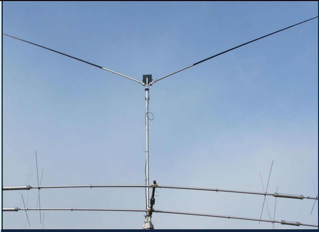
The 30m dipole is mounted about 10ft above the mini-beam
