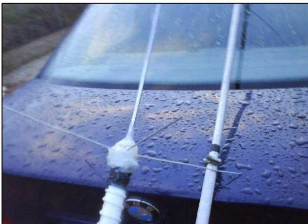
Photograph showing the four spoke of the "Top-Hat" capacitor . The joint to the antenna wire is protected with silicone bath sealant.
